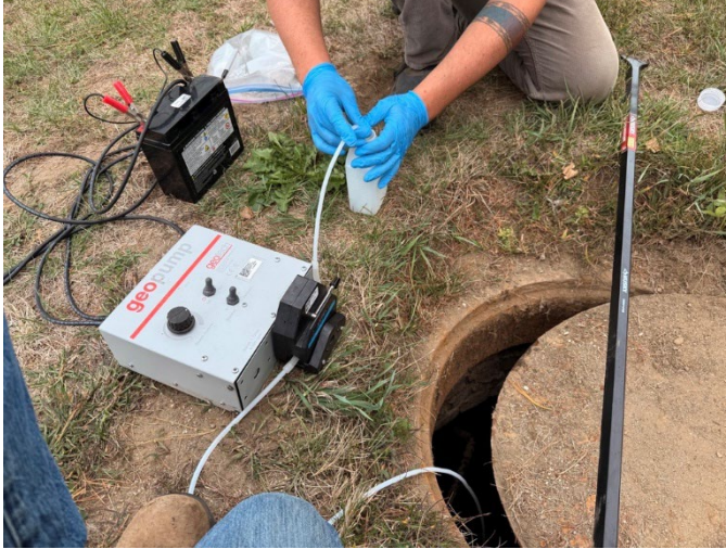
Collection of stormwater sample
