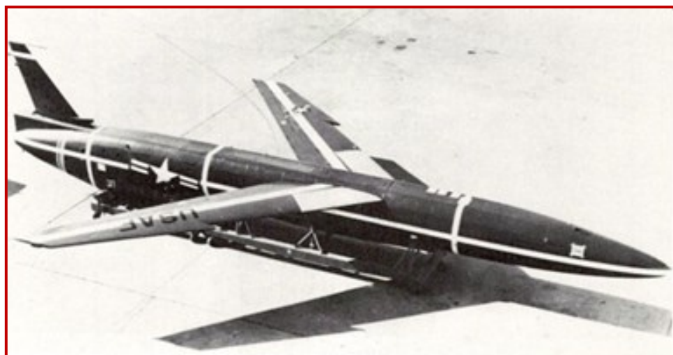
Northrop designated the enlarged Snark , N-69. Note the "saw tooth" leading edge and straight trailing edge on both the wing and the shadow of missile N-3268.
