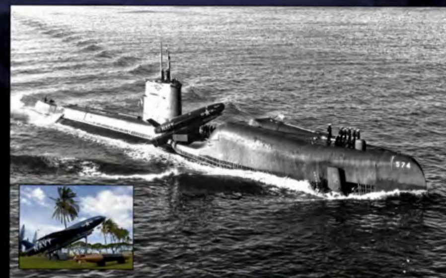
USS Grayback (SSG-574) transits the Pacific Ocean with a Regulus missile. (insert) Today, a Regulus missile sits on display at PMRF.
