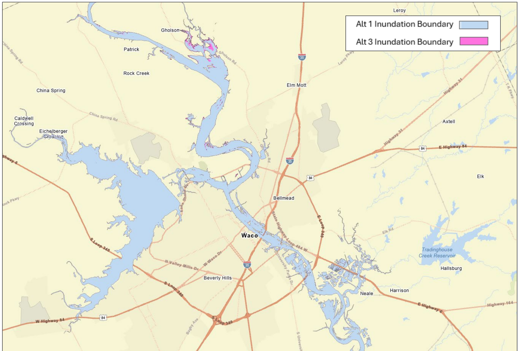
Figure 4-3: Inundation Map for the City of Waco, Frequency Analysis
