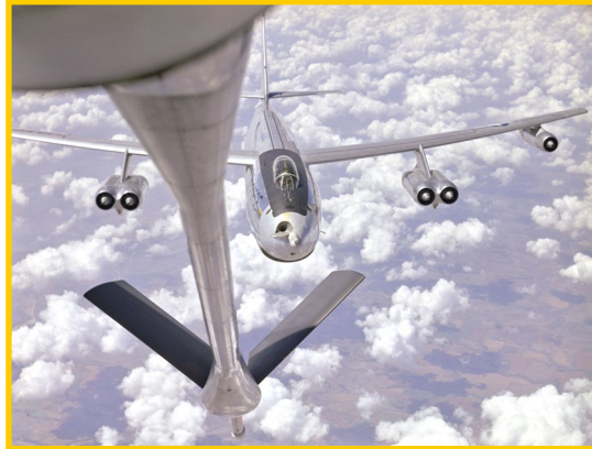
A B-47 Stratojet pulls in behind the KC-135 Stratotanker to take on fuel. Boeing Historical Archives.
