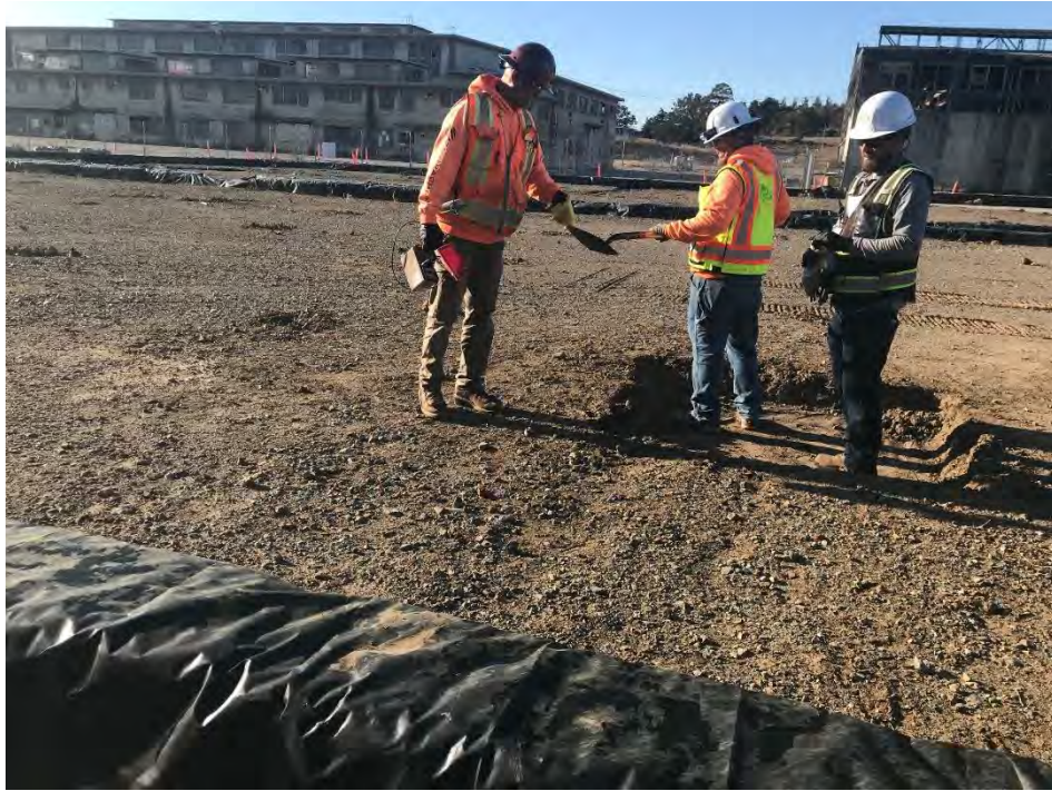
Figure 3 – Shovel being surveyed with Masslinn sheet and Ludlum 2360 w/43-93 instrument
