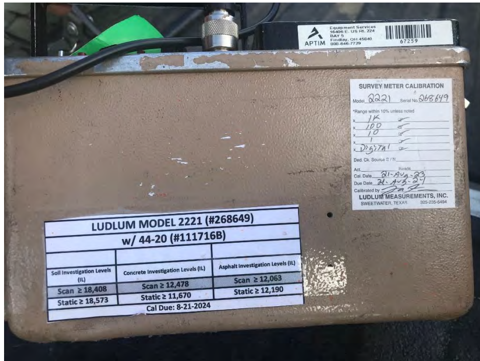
Figure 1 – Ludlum 2221, serial #268649, calibration due date 8/21/2024
