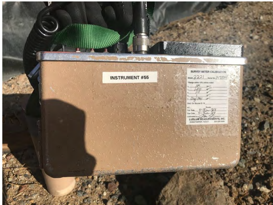
Figure 7 – Ludlum 2221, serial #147504, calibration due date 7/4/2024
