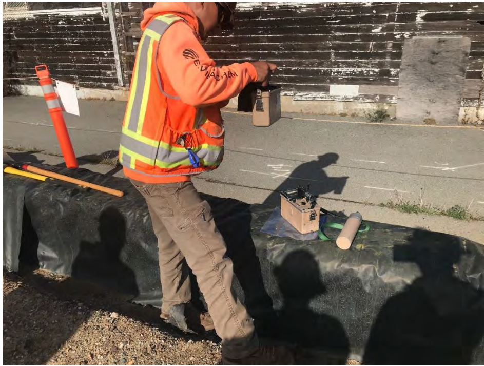
Figure 5 – RCT collecting an exposure rate measurement at 30 cm from the LLRO
