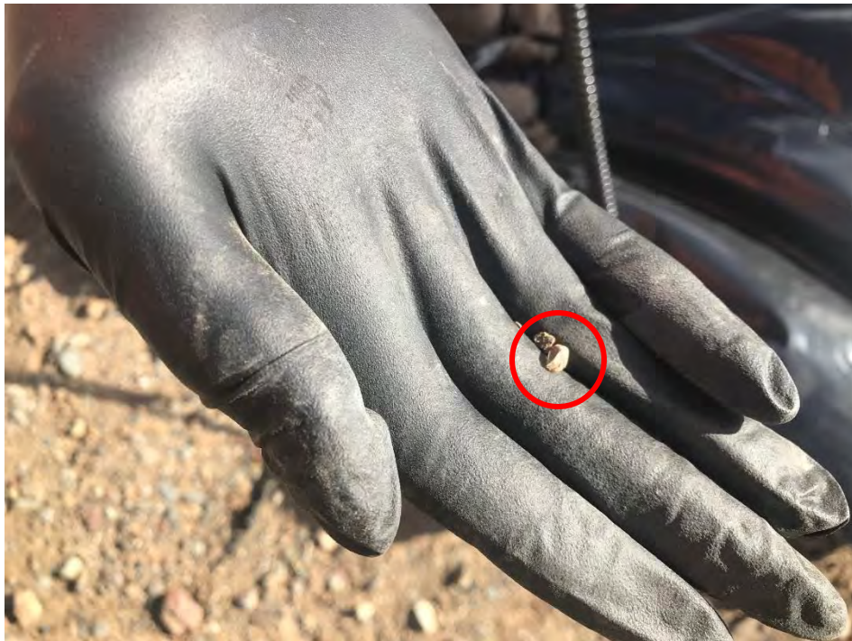
Figure 4 – LLRO was identified to be a glass fragment (circled in red)
