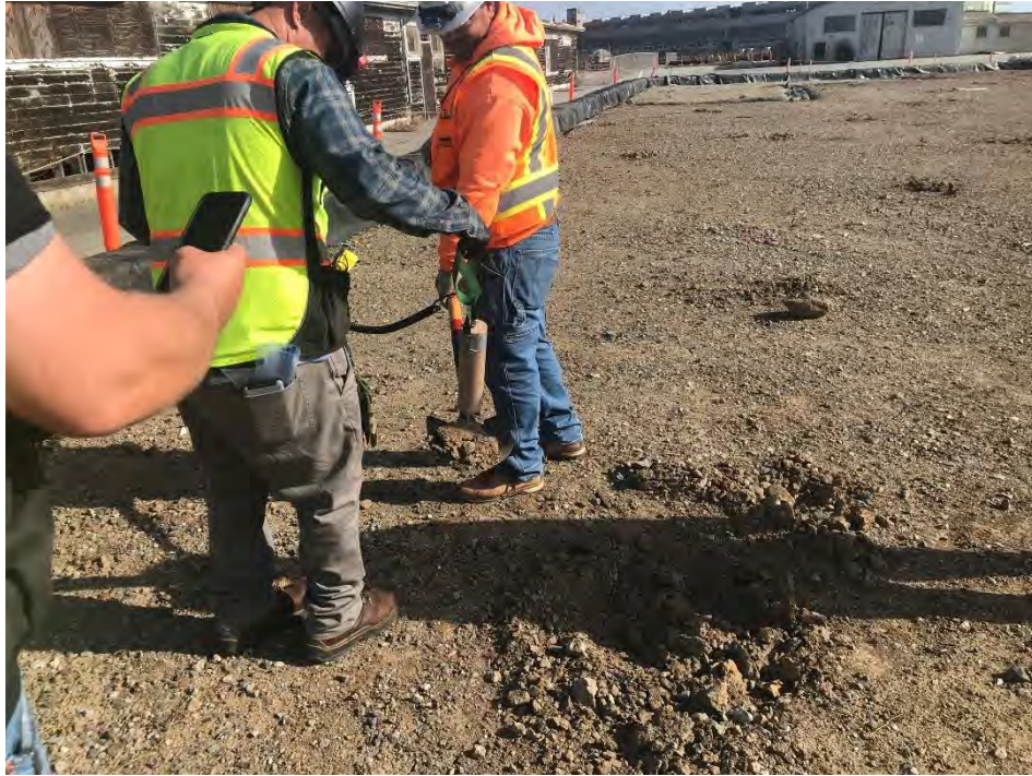
Figure 3 – Ludlum 44-10 detector used to identify and segregate the LLRO from the soil
