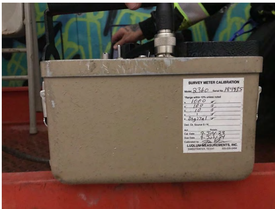
Figure 3 – Ludlum 2360, serial #184935, calibration due date 7/9/2024
