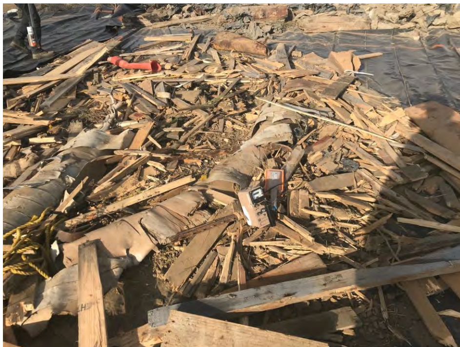
Figure 1 – 2-minute alpha/beta static measurement in progress
