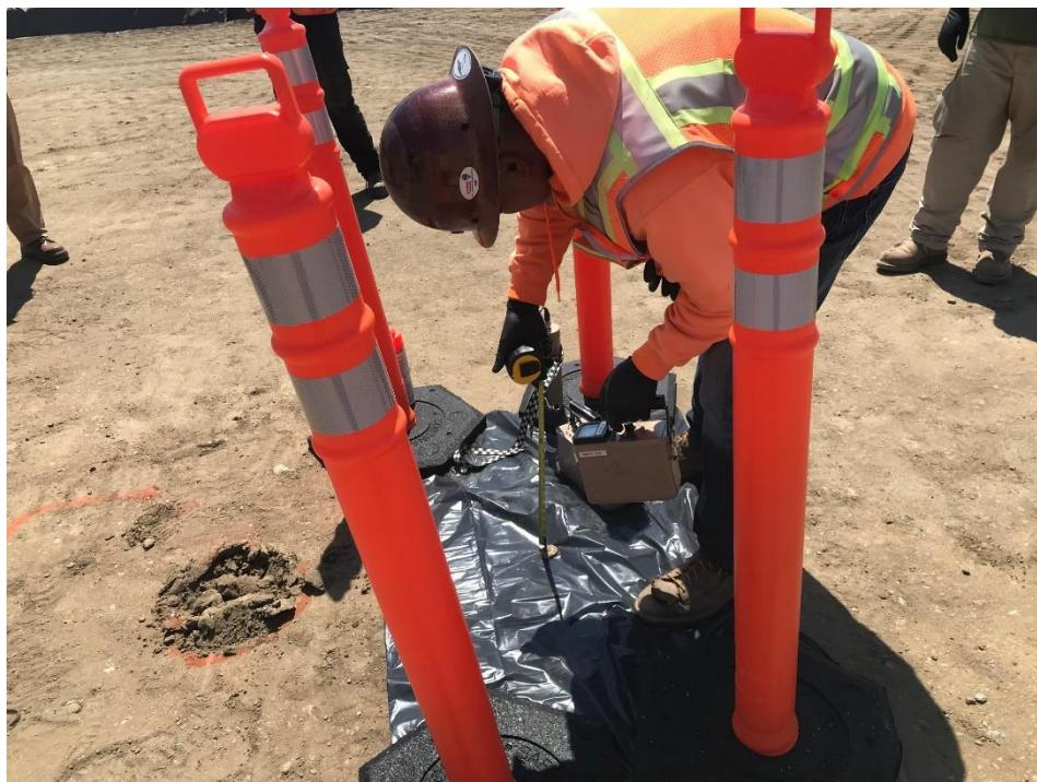
Figure 7 – Exposure rate measurement performed 30 cm away from the LLRO
