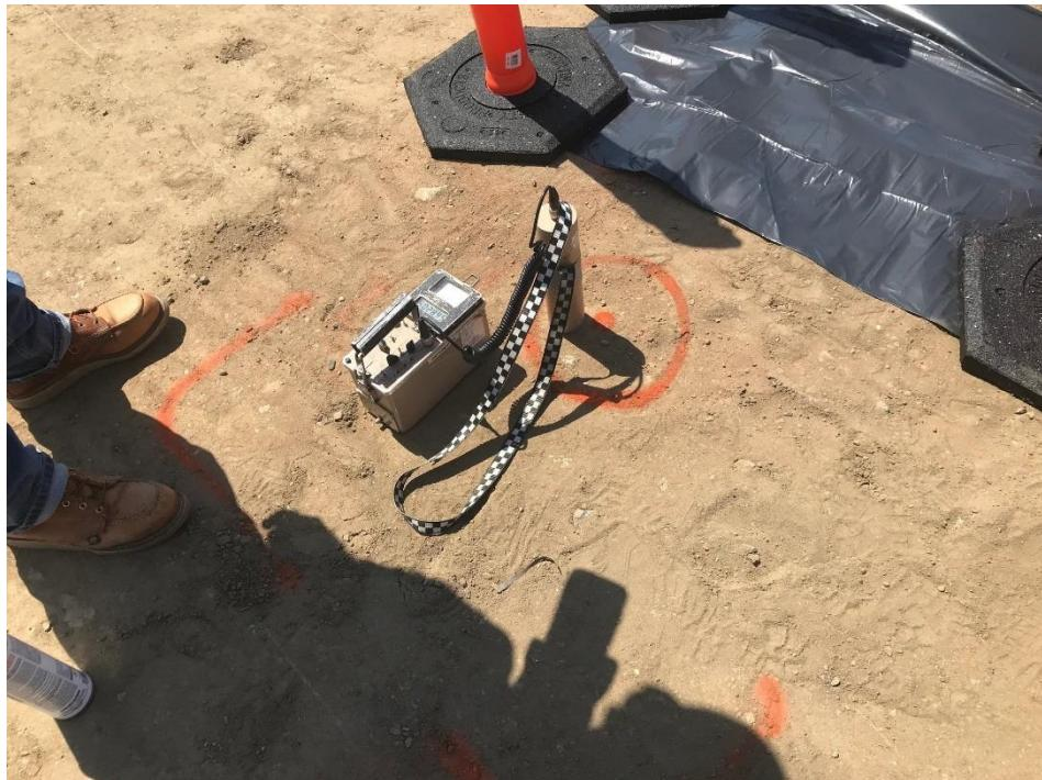
Figure 2 – Gamma static measurement performed on contact of the soil surface
