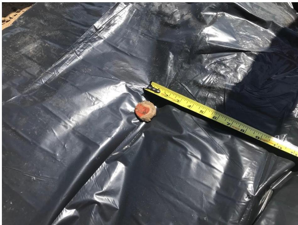
Figure 5 – A 2-inch disc shape deck marker was identified from the extraction
