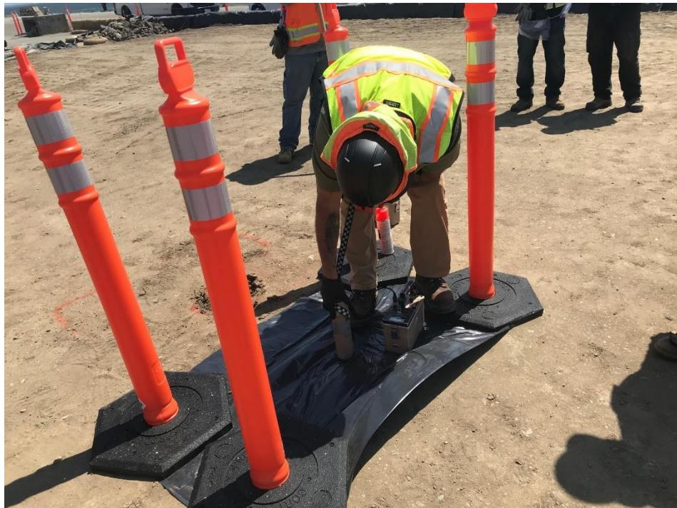
Figure 6 – Gamma static measurement performed on contact of the LLRO
