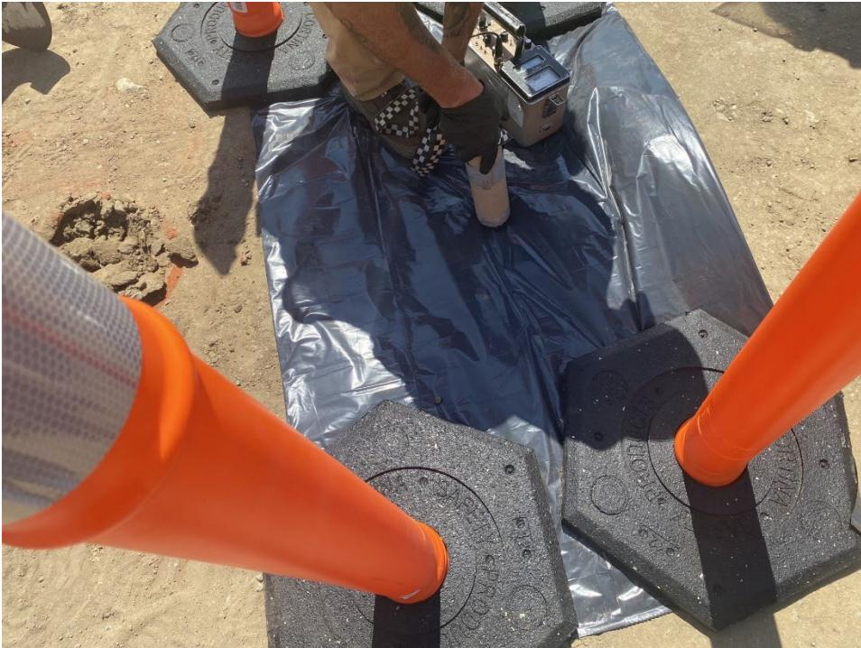
Gamma Static Count on Contact
