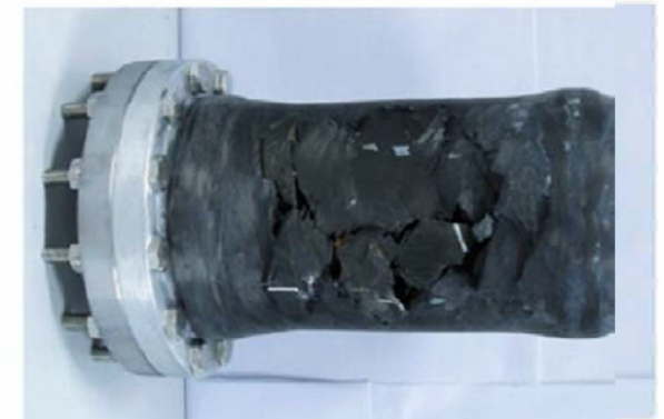
Figure 3. Hydrostatic damage test of carbon fiber composite pressure hull with aluminum liner
