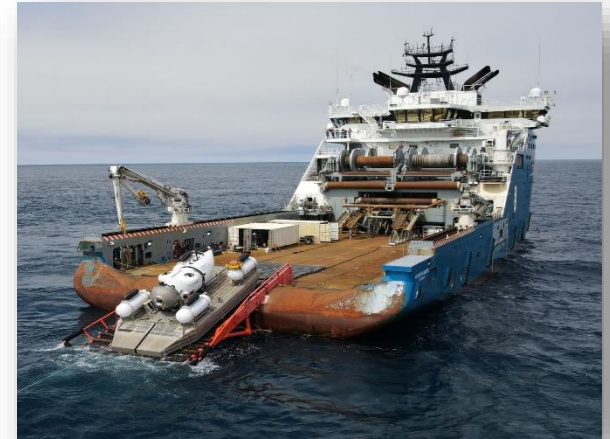
Expedition 2022, TITAN on LARS on stern ramp of the HORIZON ARCTIC, LARS/TITAN could be winched on deck during transits,
