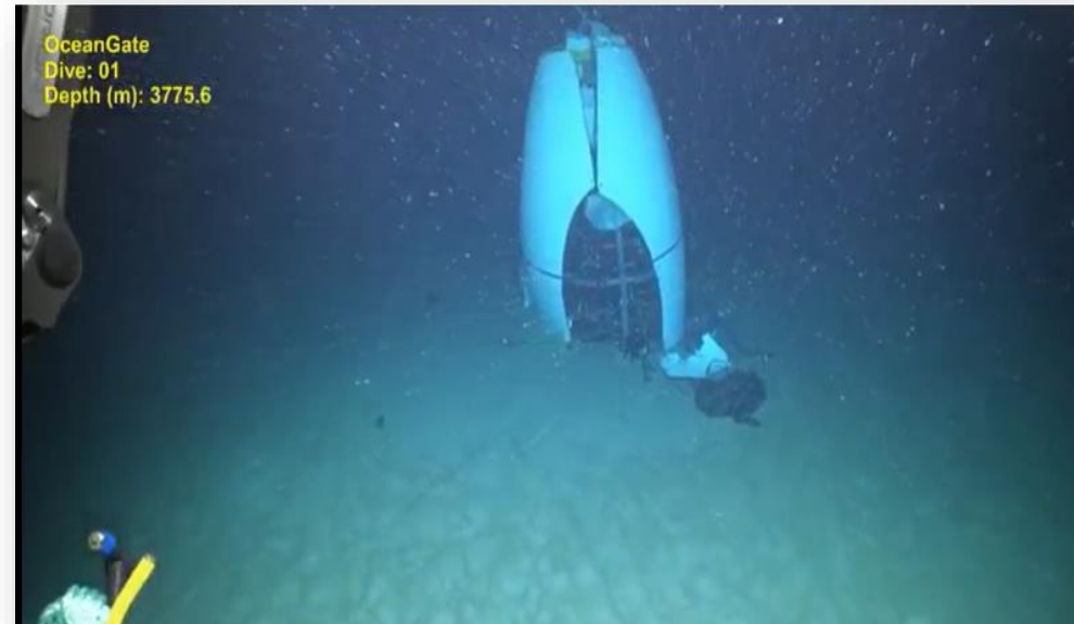
ROV image of TITAN tail cone. Source: Pelagic Research Services, June 2023
