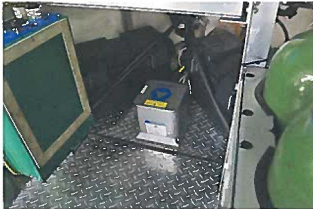
Images depicting location and size of integrated PHINS system within Cyclops 1.
