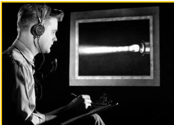
Shock waves of a thrust augmentation bleed off J-33 engine. (NASA photo)
