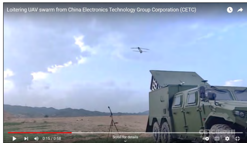
Figure 4 The launch vehicle, with 48 cells for drones. Click on picture to access video.
