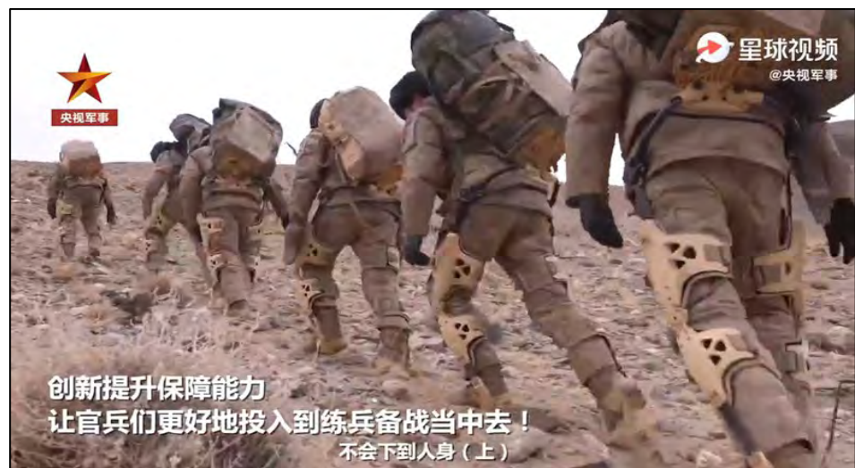
Figure 1 China powered skeleton suit for carrying ammunition for delivery in Tibet Autonomous Region.
