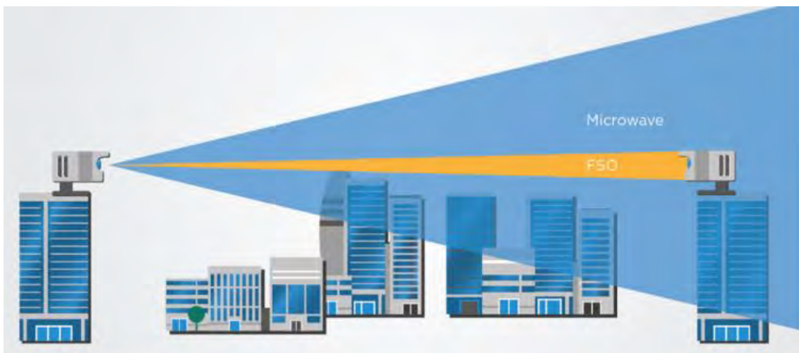
Figure 1 Image shows the comparison of signal dispersion between laser and microwave. Effect Photonics
