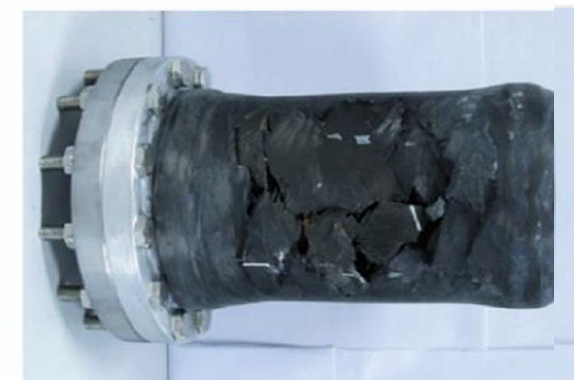
Figure 3. Hydrostatic damage test of carbon fiber composite pressure hull with aluminum liner
