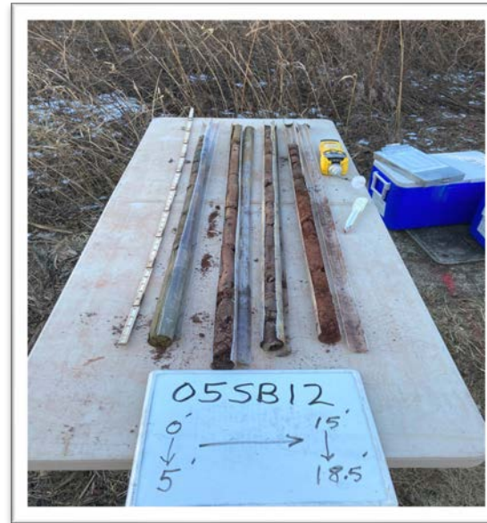
Example Of Soil Sampling Source: Tetra Tech
