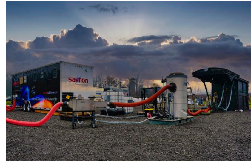
Photo from Savron's of their Ex Situ Soil Smoldering Combustion Platform
