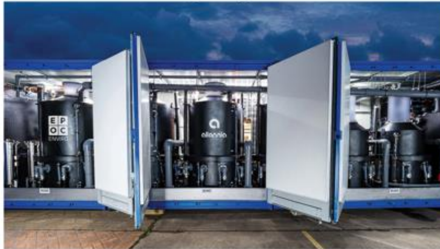
Picture of SAFF40 Unit courtesy of K. Sorenson - Allonnia
