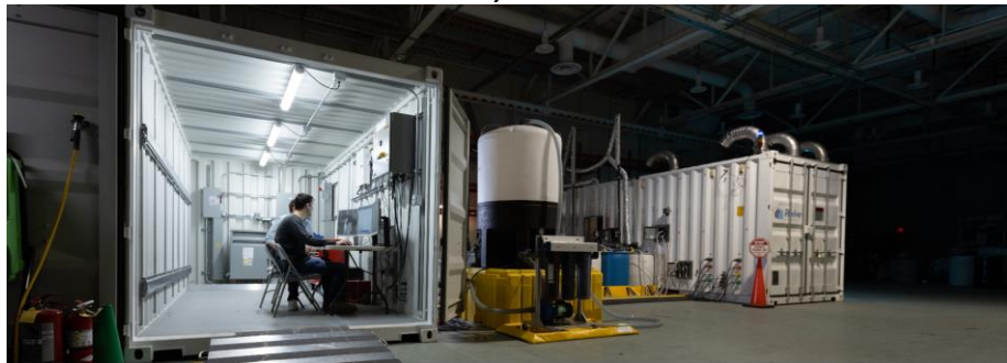
Photo Courtesy of Stephen Rosansky (Battelle) of Revive Environmental's PFAS Annihilator SCWO System
