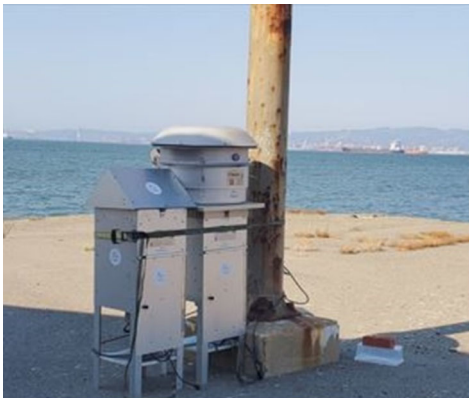
High Volume Air Sampling Stations upwind and downwind
