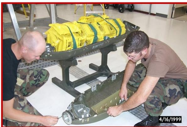
Installing det cord on the canister. (USAF)
