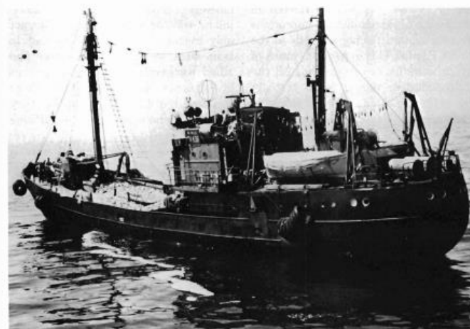
Figure 6.—Small side trawler of SRT class engaged in fishery for Pacific hake off Oregon, July 1966. Note catch of hake in forward deck bins and fish strung up to dry aft of wheelhouse. Fenders of tires are used when alongside another vessel.
