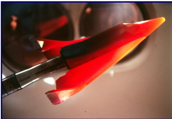
The effects of aerodynamic heating show up well on this model of Dyna-Soar during a 1962 test in the von Karman Facility (VKF) at Arnold Engineering Development Center, TN. (AEDC History Office)
