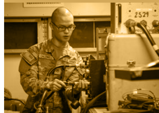
U. S. Army Private First Class Joseph Caldwell, a Next Generation Automatic Test System (NGATS) Operator assigned to B Company, 299th Brigade Support Battalion, 2nd Armor Brigade Combat Team, 1st Infantry Division, diagnosing line replaceable units (LRUs) for Abrams battle tanks and Bradley infantry fighting vehicles on Fort Riley, Kansas, April 26, 2024. (Photo by Sfc. David L. Edge)
