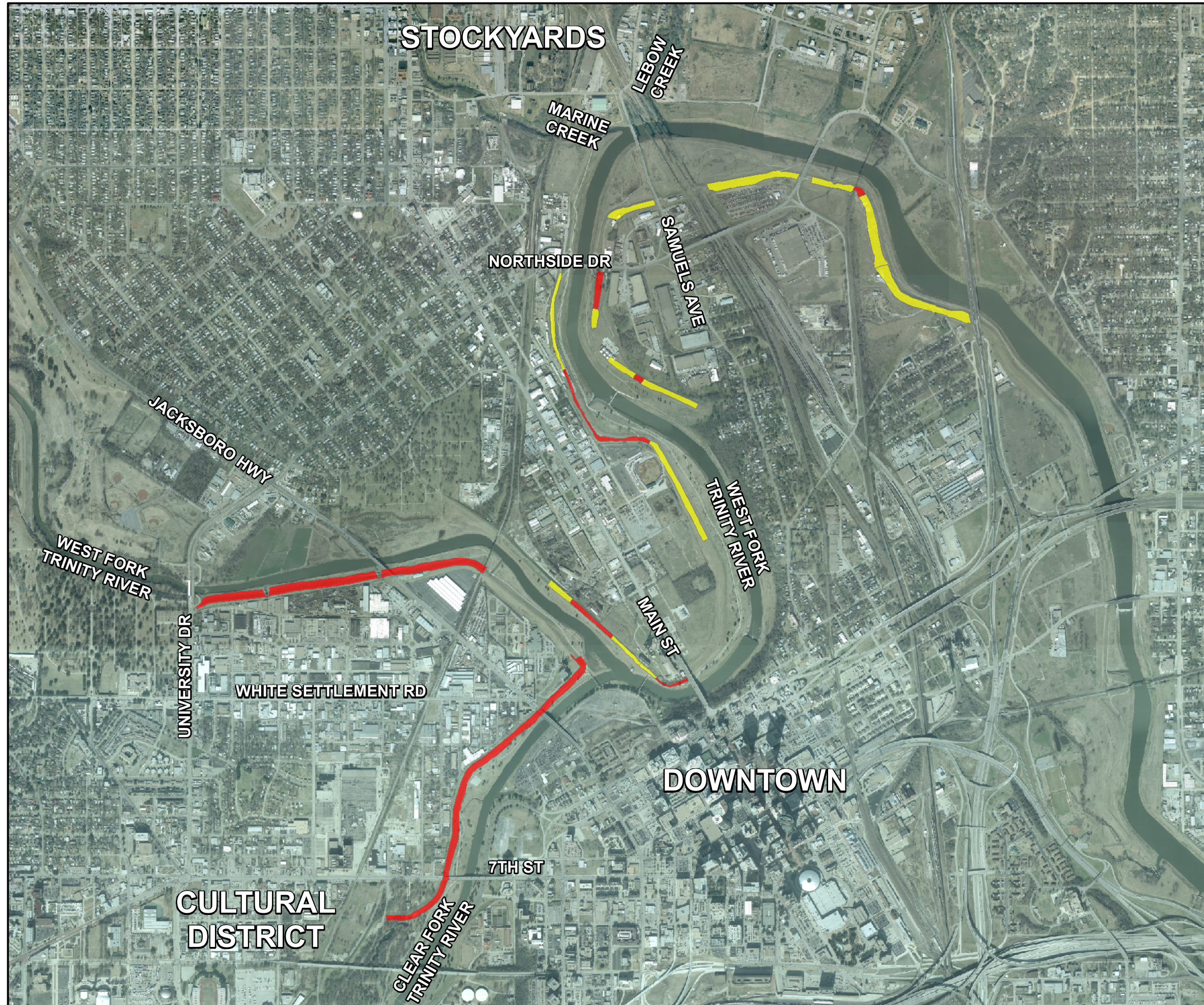
Central City Figure 2-3. Deficiencies of the Existing Levee System in Comparison to Design Criteria
