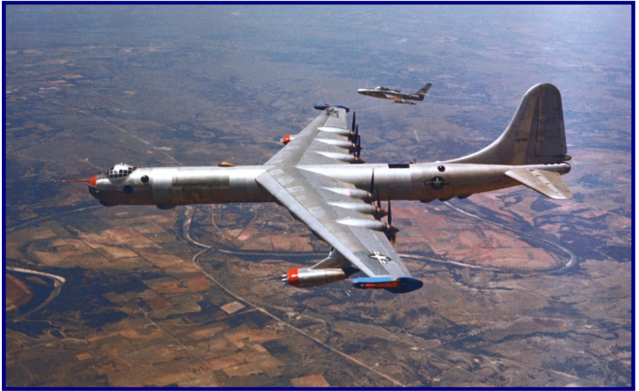
A Republic RF-84F pulls up to the right wingtip of this JRB-36F during a test mission under Project Tom-Tom. (AFMC History Office)
