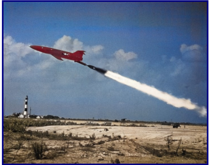
A colorful Martin Matador launches from the Eastern Test Range of the Air Force Missile Test Center, FL. The bright colors made the missile easier to track during test missions over the Atlantic Ocean. (AFMC History Office)
