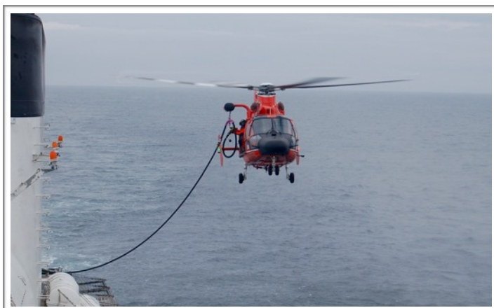
The helicopter is fueled while flying in an evolution called a HIFR.
