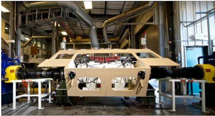
Bradley Fighting Vehicle undergoing hybridization retrofit
