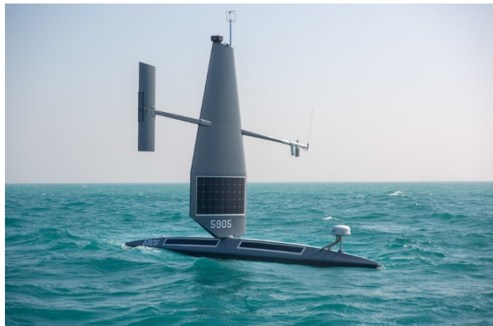
"Saildrone wing" combines wind and solar panels for propulsion.
