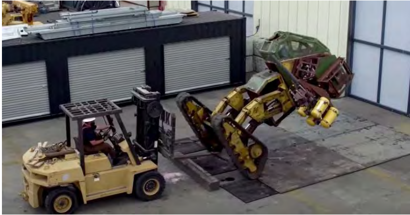
"MegaBots" tests the durability of its giant robot with a crash test. The top-heavy robot easily tips over. (Video screenshot by Bonnie Burton/CNET)
