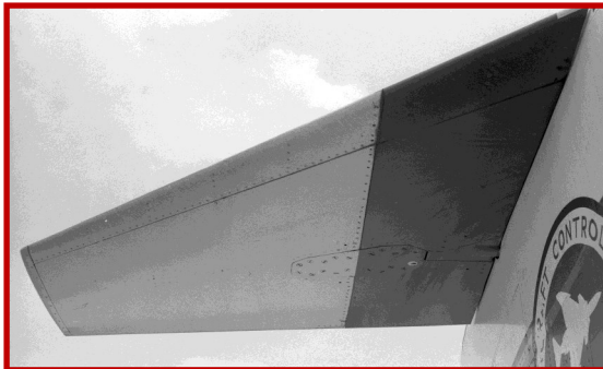
The removable, white-painted, outer portion of the canards show up well in the underside view above. (Author)
