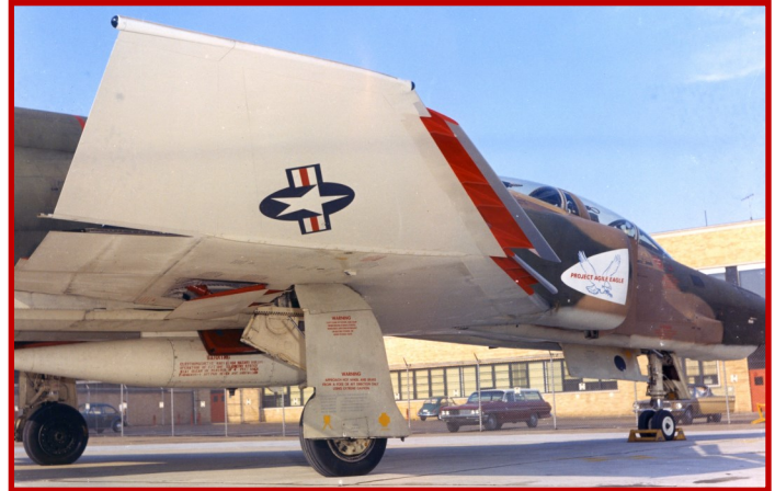
The fixed wing leading edge slats show up well in this view of 12200 during Project Agile Eagle IV. (Boeing Historical Archives)
