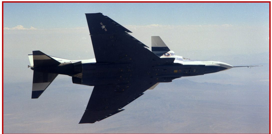
The YF-4E, with canards and wing leading edge slats installed, banks away from the camera during a test mission on 18 July 1974. (AFTC History Office)
