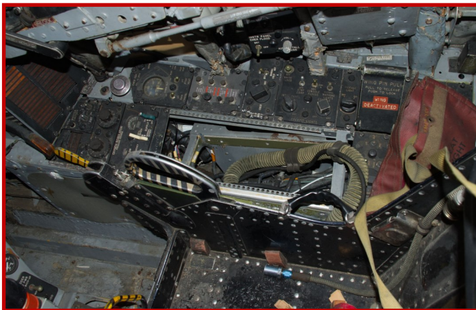
Fair quality illustration showing the modified forward cockpit of YF-4E #62-12200 during the PACT/CCV test program. Note the side stick control on the right hand console in the cockpit, and canard control switches on the left side of the main panel and left console. (USAF)
