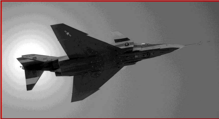
The dark blue bottom (FS 15044) and lack of wing leading edge slats show up well in these 2 flight views of the YF-4E over Edwards AFB on 12 August 1974 at left. (USAF Photos by Sgt. Wayne Berry-AFTC History Office Collection)
