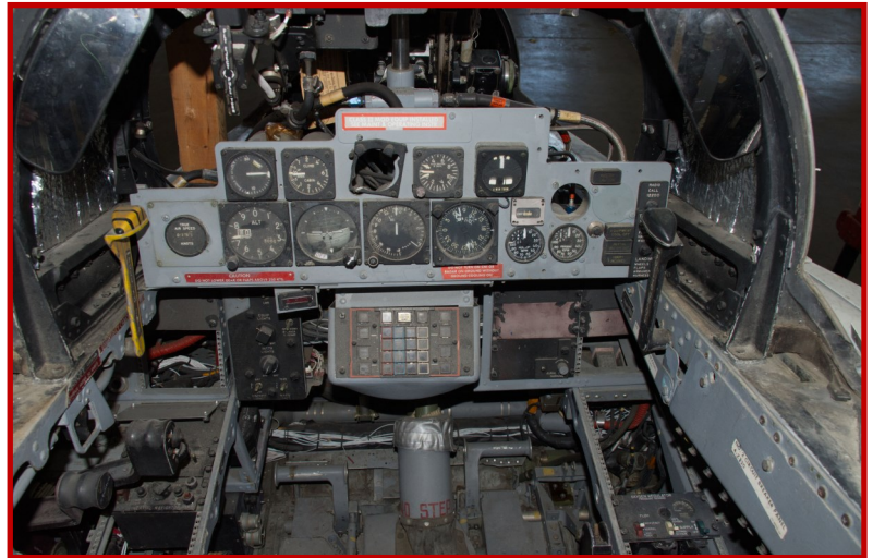
The YF-4E aft cockpit (above) contained basic flight instruments as the aircraft could be flown from this position. The back-up SFCS/Fly-By-Wire control display is beneath the flight instruments, and the aft side stick control has also been removed. (Author)
