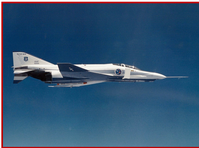
The YF-4E during a test flight out of Edwards AFB, CA. The aircraft is carrying the McDonnell Douglas Eliminate Range Zero System (EROS) collision avoidance pod in the aft left missile bay. (AFTC History Office)
