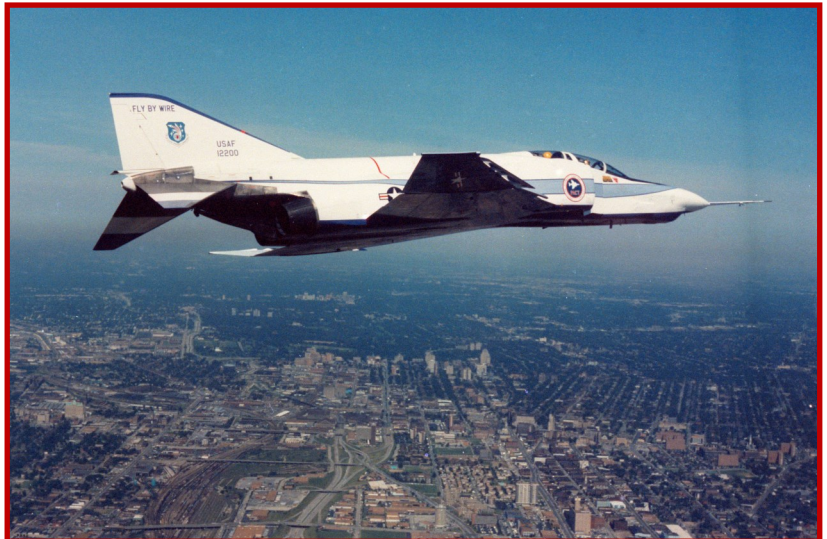
The canards mounted on the shoulders of each intake have a span of 5 feet with a surface area of 17 square feet. The outer 3 feet of each canard is removable and a single test flight was accomplished utilizing the partial-span canards. (USAF Illustrations)
