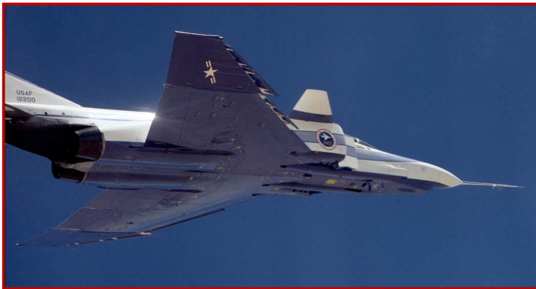
The wing leading edge slats and canards show up well in this underside view of the YF-4E taken on 5 July 1974. Note the addition of the PACT emblem on the right side inlet. (AFTC History Office)
