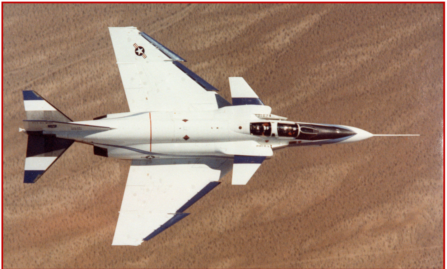
Stunning over-the-top view of YF-4E 12200 during a test flight over the Mojave Desert during the PACT test program. The canards on each intake and the addition of fixed wing leading edge slats show up well in this view. (AFTC History Office)
