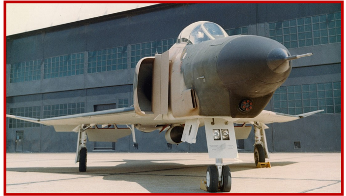
After McDonnell installed the M61A1 Gatling gun in the nose, the aircraft was known as the 'F-4-TFS'. (Mark Nankivil Collection)
