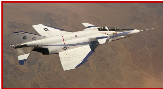
McDonnell Douglas/AFFDL YF-4E fly-by-wire testbed in flight near Edwards AFB, CA. (AFTC History Office)
