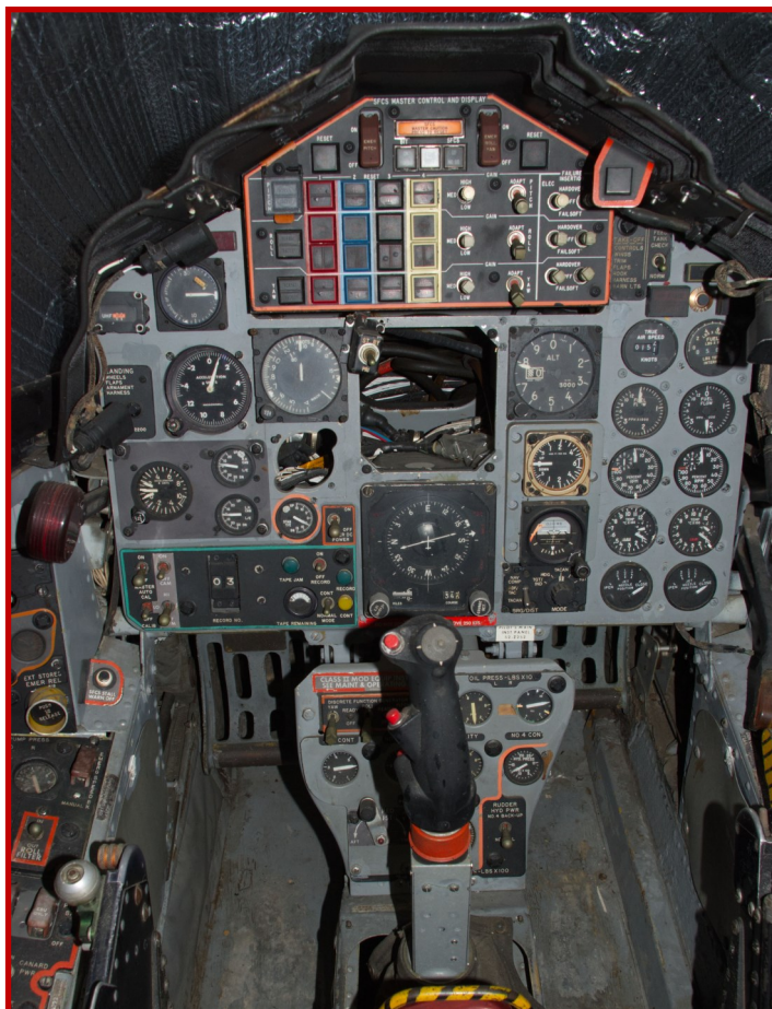
The heavily-modified cockpit of the YF-4E remains mostly complete as of July 2024. The SFCS/Fly-By-Wire control display occupies the majority of the instrument control panel (above). Unfortunately, the side stick control had been removed from the right side console (left) prior to coming to the museum. (Author)
