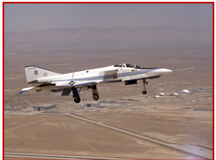
Gear down & flaps deployed, the flight test crew of YF-4E #62-12200 prepares to make a left turn approach to the main runway at Edwards AFB. (AFTC History Office)
