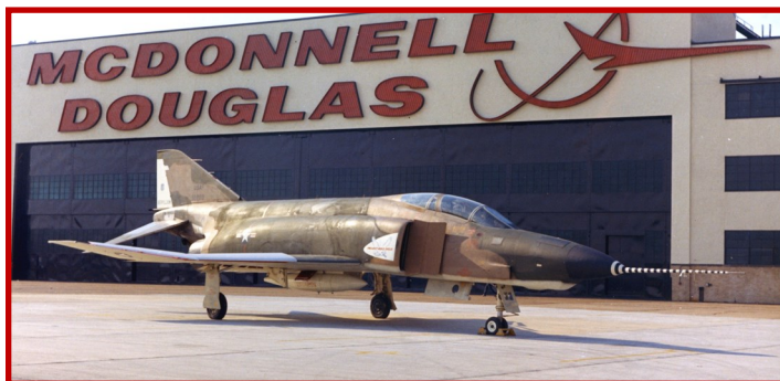
The next step in the evolution of the YF-4E was the testing of a Beryllium rudder and wing leading edge slats during Project Agile Eagle. (Boeing Historical Archives)
