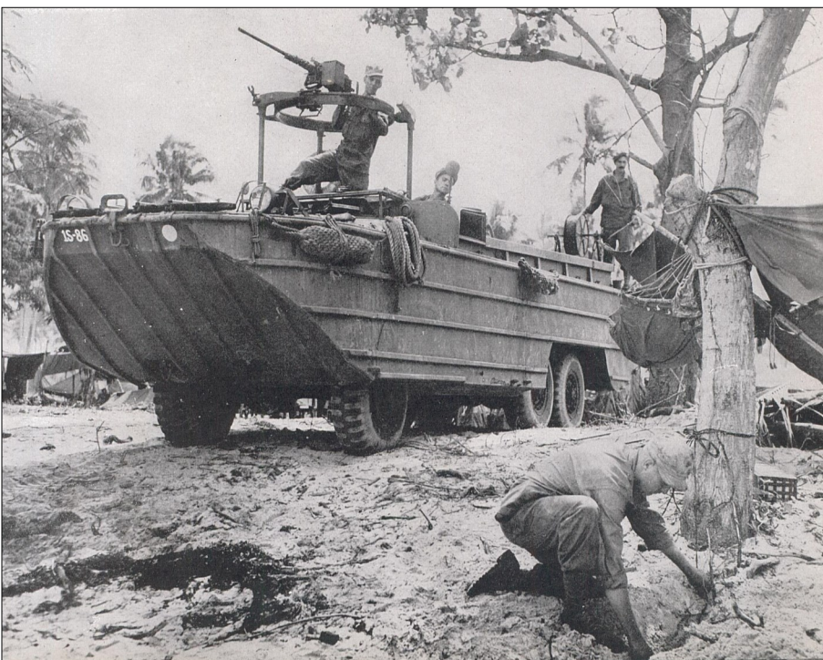
Soldiers of 1st Signal Troop emplacing wire using a DUKW amphibious vehicle at Los Negros Island. (Photo from Signal Historical Collection)
