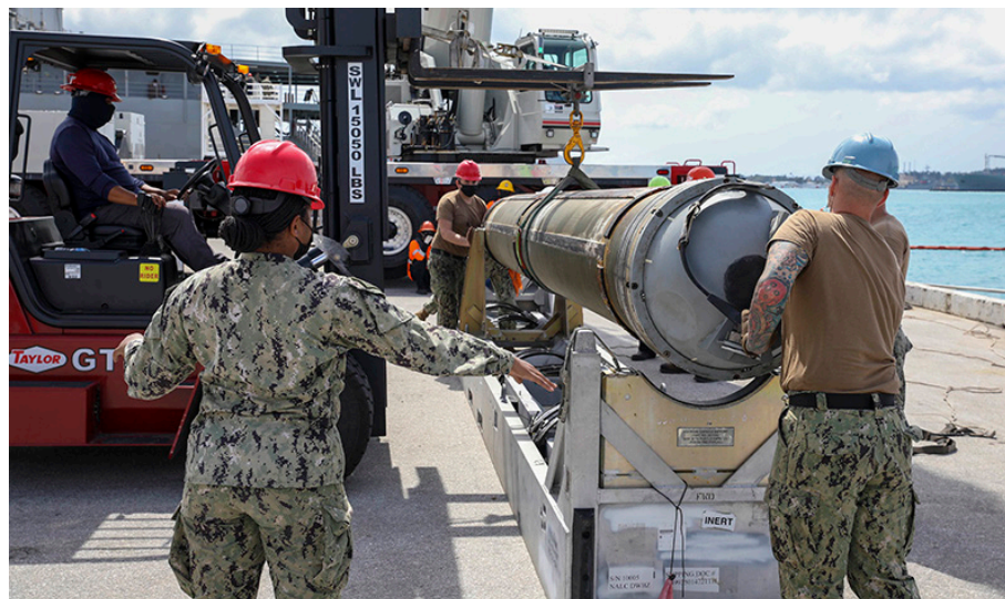
Sailors assigned to the submarine tender USS Emory S. Land (AS 39) weapons handling division conduct an offload of a Tomahawk missile from the Los Angeles-class fast-attack submarine USS Asheville (SSN 758), February 1, 2022.
