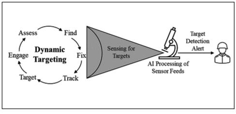
Figure 4. Al augmentation of targeting: Al can augment the dynamic targeting cycle by searching for targets and then sending alerts upon detection
