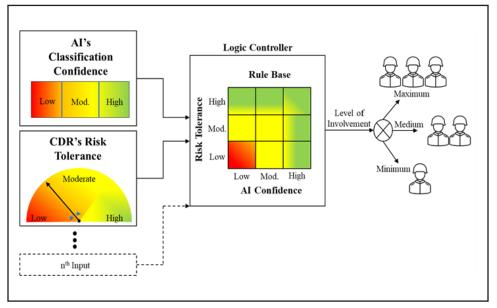
Figure 9. Combining Al's classification confidence and CDR's risk tolerance: A block diagram for a programmable controller designed to gauge the confidence of Al and the risk tolerance of the commander for every newly detected target and then choose the level of oversight under which the targeting process should occur
