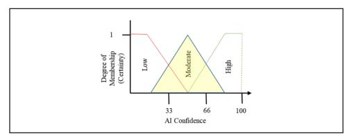
Figure 7. Fuzzy logic: An illustration of possible fuzzy sets for the input AI Confidence. The shapes of these fuzzy sets are designed by a human using expert knowledge.
