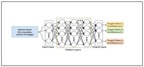
Figure 2. Deep neural networks (DNNs) and targeting: Concept diagram of DNN used in target detection. In this case, as new images are captured from a sensor, they are processed through the DNN, which predicts, with a degree of confidence, whether a particular target exists in the image.
