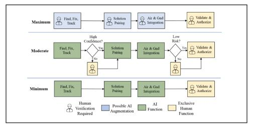
Figure 10. Risk profiles: Three risk profiles for varying the level of human oversight in an AI-enabled targeting process based on conditions assessed by a fuzzy-logic controller
