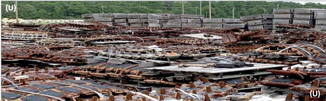
(CUI) Figure 5. Vehicular Track Shoes Stored Outside at [REDACTED] Without Any Packaging (U) Source: The DoD OIG.
