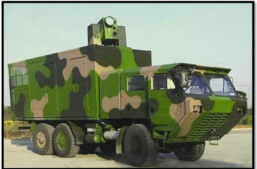
Figure 15: LAG II Mobile, Ground-based laser potentially capable of shooting down drones, artillery shells, and missiles. Source: globalsecurity.org
