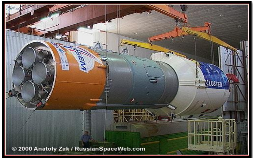
Figure 73 Stage III of the Soyuz rocket attached to its payload Russian Pace Lab
