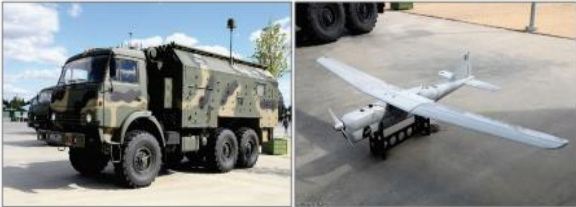
Figure 37: Drone based Jamming. The Leer-3 Command Vehicle and Orlan-10 type EW drone. Source: Vitaly Kuzman. Can view at: http://dl.icdst.org/pdfs/files3/906f2544ddd693eb1118881a5baff0a3.pdf
