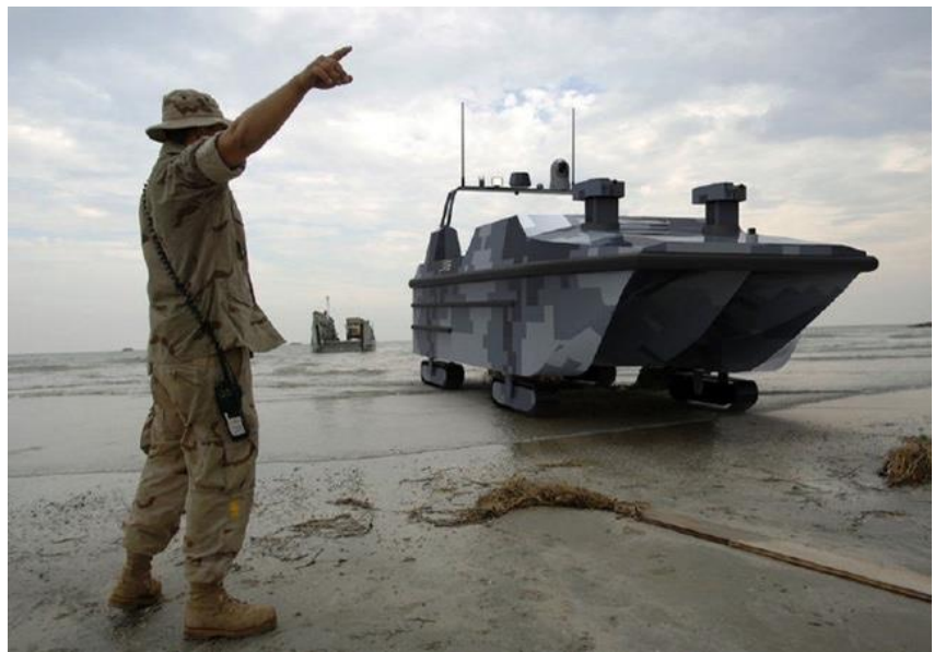
Figure 13: China demonstrate the transition of domain from sea to land in a prototype of an autonomous landing craft. Source: The Verge
