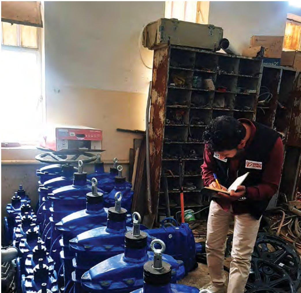
A Mercy Corps staff inspects gate valves during the Water, Sanitation, and Hygiene activity rehabilitation of the Al-Ghilzane Water Treatment Plant, Mosul, Iraq. (USAID photo)
