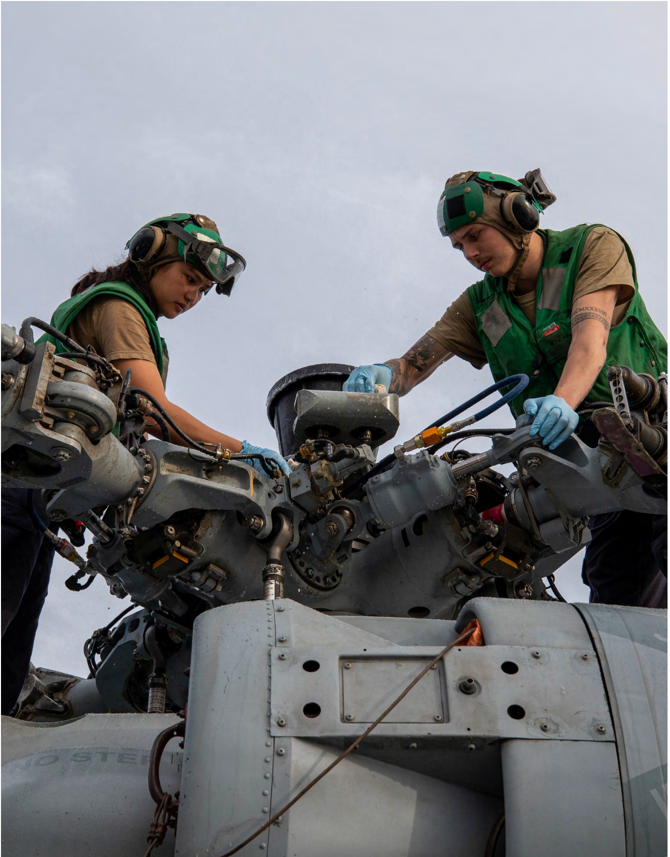
A Sailor and Airman clean the spindle of a MH-60R helicopter aboard the guided missile destroyer USS Roosevelt in the Baltic Sea. Source: U.S. Navy.
