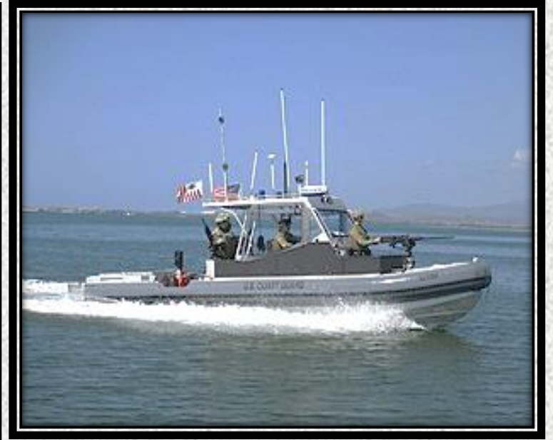
32-foot PSU - TPSB Partially enclosed cabin Hardtop cover Utilized in present day for “Defense Readiness Operations”
