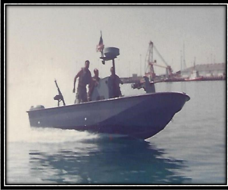
22-foot PSU - TPSB Open Deck No cover Utilized in 1991 Gulf War “Desert Shield - Desert Storm”
