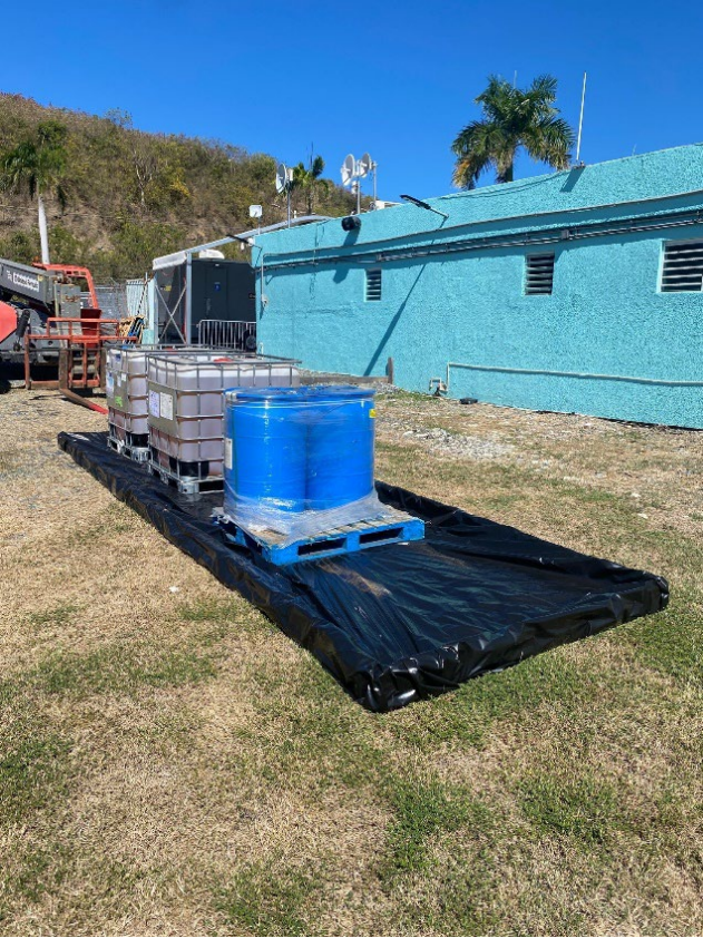
EVO Totes and Drums w/in Secondary Containment
