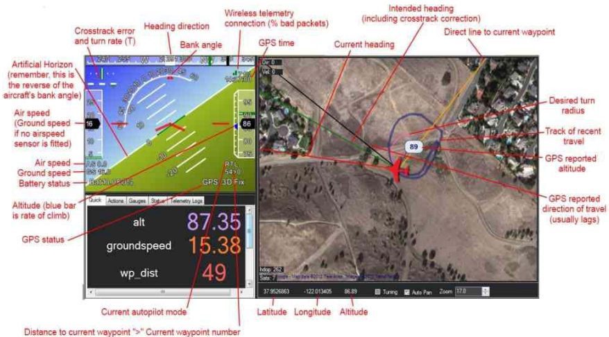
Figure 2-9. A Modern Autopilot Control, an Ardupilot Ground Control Station. 15
