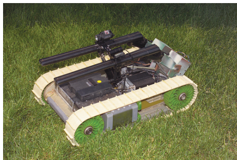
The Rapid Equipping Force's PackBot with "teeth" (shotguns).
