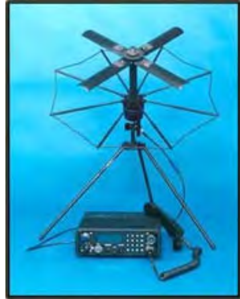
Figure 13: Tactical Satellite Radio and Antenna
