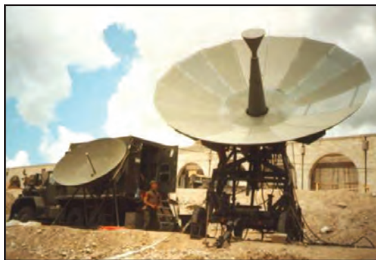
Figure D-13. AN/TSC-85B/C Shelter.
