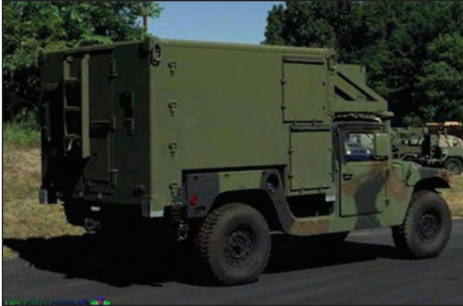
Figure D-18. Single Shelter Switch AN TTC 56
