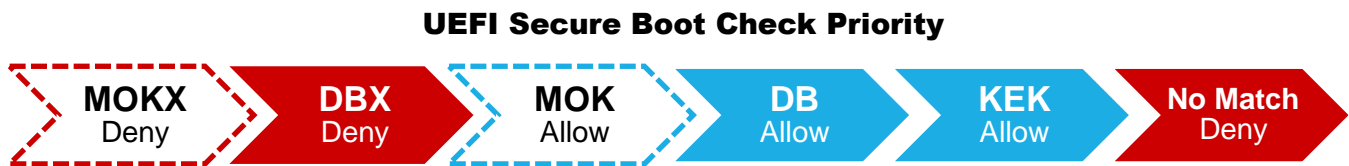
Figure 2 - Order of operations during UEFI Secure Boot checks. Checks contained within dashed lines only take place when the Shim bootloader is used AND after its initialization in the UEFI bootloader phase (i.e. firmware OROMs are not checked against MOKX and MOK; kernels are checked against MOKX and MOK).
