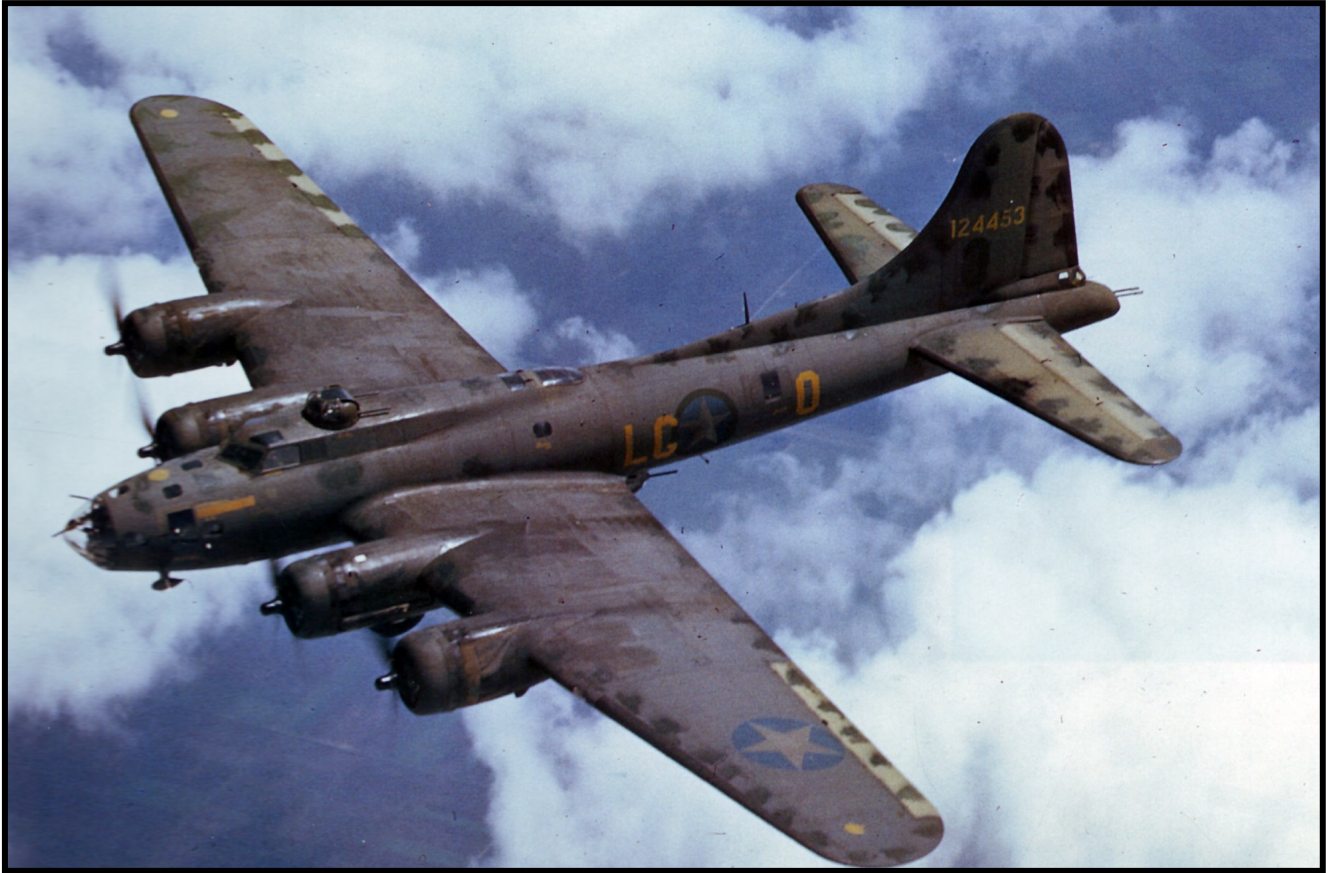
Above: Boeing B-17F of the 8th Air Force in standard Olive Drab finish with Medium Green “splotches” on the upper surfaces. The Olive Drab paint, while effective, also faded quickly in service due to wear and sunlight exposure. Also note the difference in shade between the metal skin of the aircraft and the fabric-covered ailerons and elevators.
