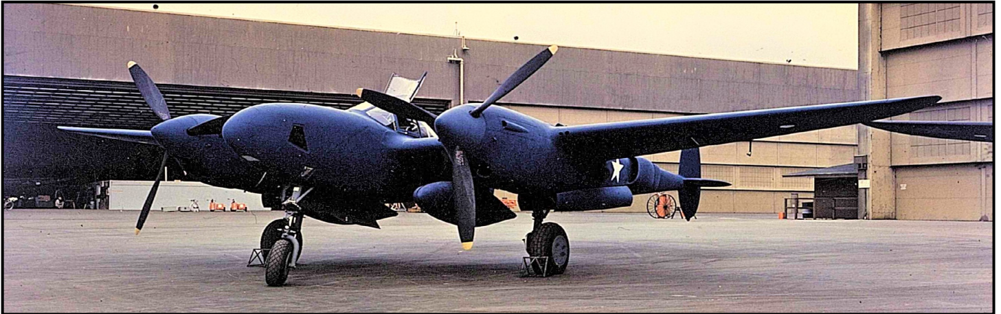
Above: Lockheed F-5 Photo Reconnaissance aircraft in Haze Paint. The use of this finish did aid concealment by allowing the aircraft to blend in with the sky at high altitudes but the design also drew attention to the fact that these were not the armed fighter version of the P-38—normally in Olive Drab or Natural Metal finish.
