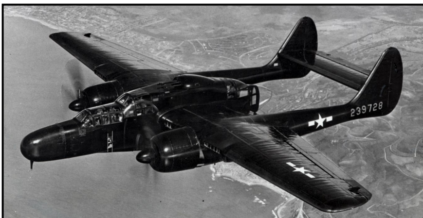
Left: Northrop P-61 Black Widow in glossy “Jet Black” finish, found through extensive testing to be the superior camouflage for aircraft operating at night. Night fighters remained in gloss black even after camouflage was removed from most other USAAF aircraft.
