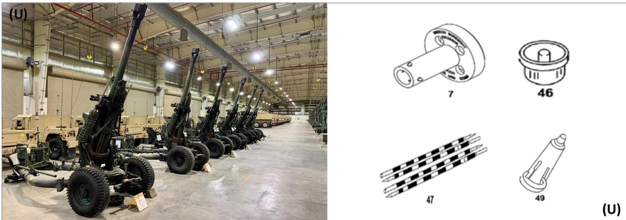
(U) Figure 1. M119A3 Howitzers and BII Required for Operation
