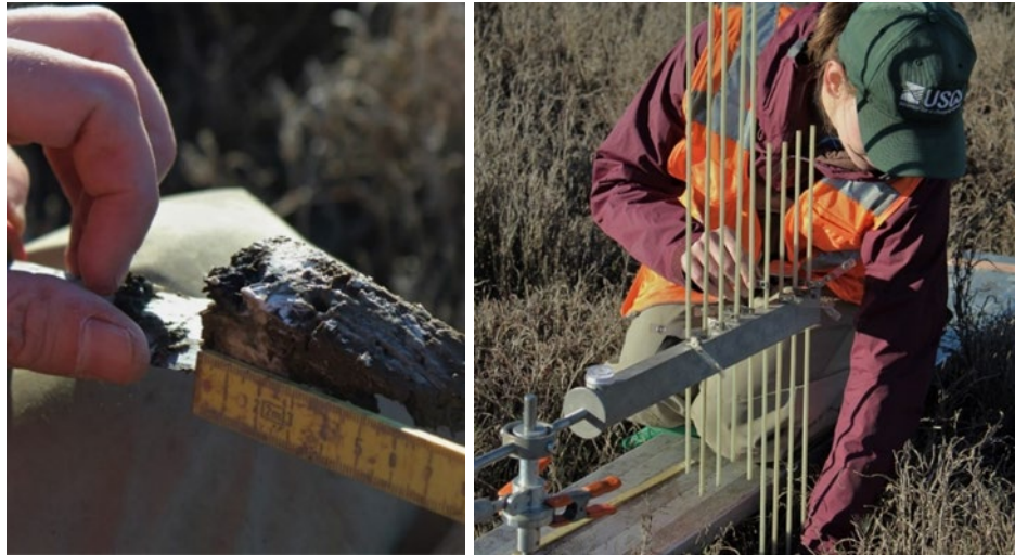
Figure 2-5. Marker horizons can be used to measure the amount of deposition that occurs in a marsh (left). The arm reader for a Surface Elevation Table (SET) can provide mm measurements of elevation change (right).
