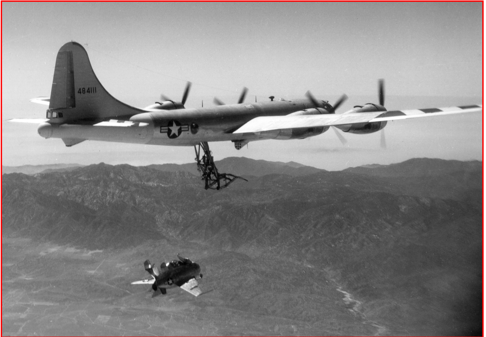
McDonnell test pilot Edwin Schoch performs the first free flight of the Goblin on 23 August 1948 in the skies near Muroc AFB, CA (now known as Edwards AFB). After 10 minutes of free flight, Schoch made two, unsuccessful attempts to hook up with the mothership before making a safe, skid landing on the lakebed below.
