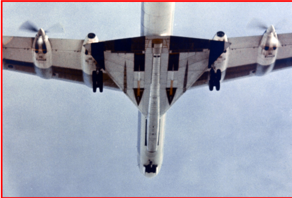
Though not exactly a parasite, the largest article carried by a B-36 was the static test airframe for the B-58 Hustler. B-36F, 49-2677, was used to take the test article from Convair's plant in Ft. Worth, TX to Wright-Patterson AFB, OH for static loads testing on 12 March 1957. Note the removal of the inboard propellers on the Peacemaker.
