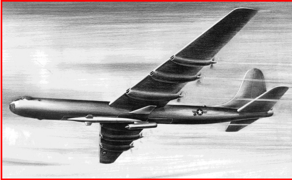
Early concepts of the North American Aviation Navaho missile system were air-launched designs such as this single-engine variant carried aloft by a B-36.
