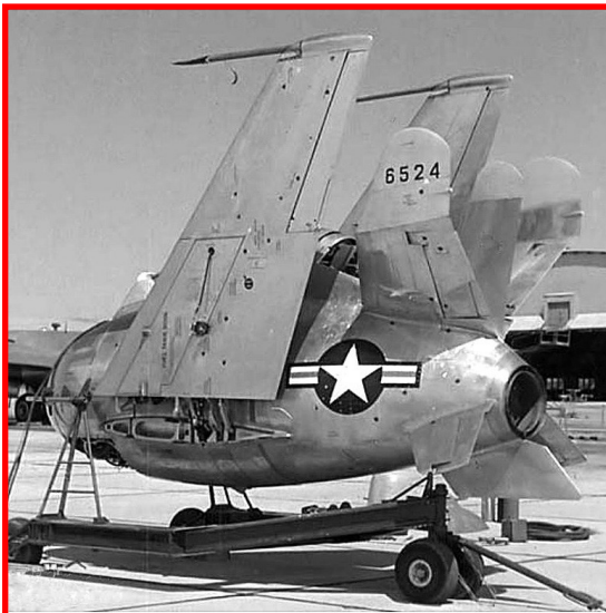
Both XF-85 airframes retained their folding wing feature despite not being utilized during testing with the EB-29B.
