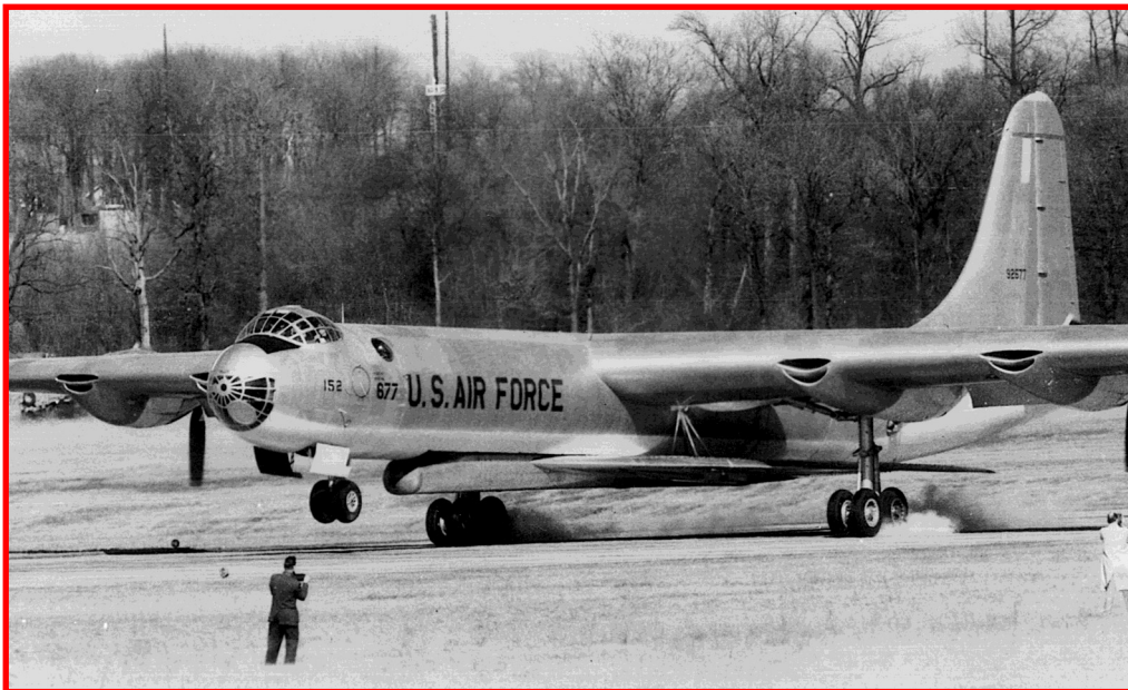
B-36F, 49-2677, carrying the B-58 Hustler static test airframe lands at Wright-Patterson AFB, OH on 12 March 1957. Convair found it safer to transport by air than by ground shipment.
