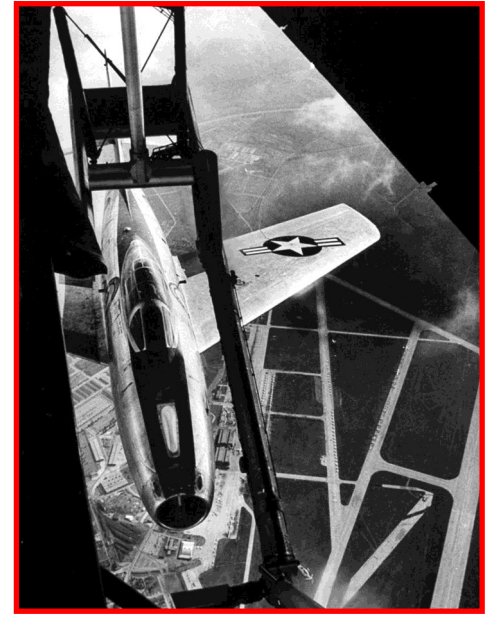
While loading operations could be accomplished on the ground, crews found it easier for the two aircraft to depart separately and mate up in flight (above, left). The RF-84K nearly always carried two external fuel tanks during normal operations. Little is known about the actual operational reconnaissance missions flown by Thunderflash crews. The view from the bomb bay during a hook-up looks pretty dramatic as shown above right during a hook-up test mission utilizing an F-84F Thunderstreak.
