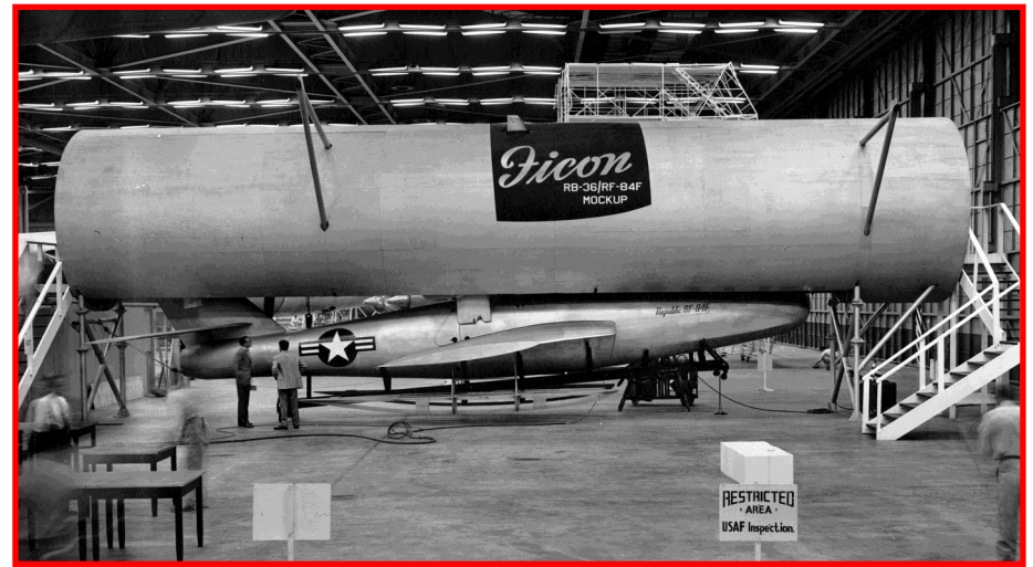
To test the FICON concept, Convair constructed full scale, wood mockups of the B-36 center fuselage as well as the Republic RF-84F. The modified aircraft were given the designations GRB-36D and RF-84K respectively.
