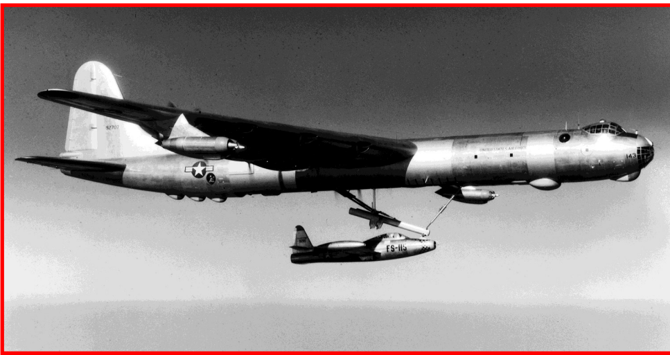
A follow-on to the XF-85 Goblin concept, Project FICON (Fighter Conveyor) made use of modified RF-84F Thunderflash aircraft, though initial testing was completed using a single Republic F-84E Thunderjet, 49-2115, as shown above.
