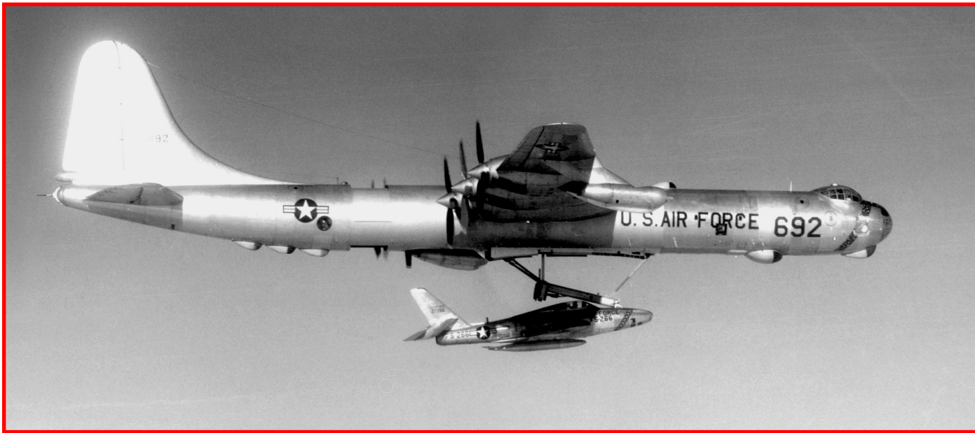
While loading operations could be accomplished on the ground, crews found it easier for the two aircraft to depart separately and mate up in flight (above, left). The RF-84K nearly always carried two external fuel tanks during normal operations. Little is known about the actual operational reconnaissance missions flown by Thunderflash crews. The view from the bomb bay during a hook-up looks pretty dramatic as shown above right during a hook-up test mission utilizing an F-84F Thunderstreak.
