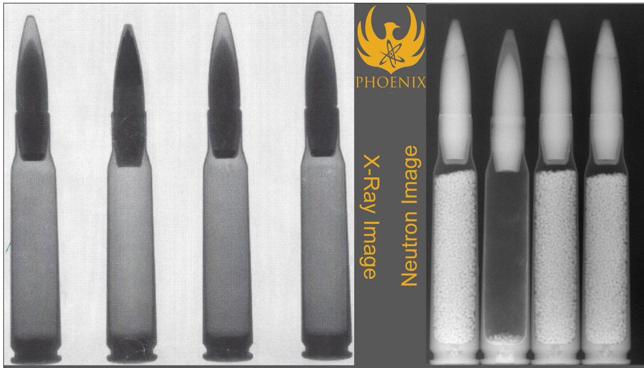
Neutron radiography, as an inspection technique, complements traditional x-ray techniques. It easily penetrates a metal shell to reveal the lighter materials inside.
