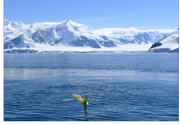
Deployed from the Rothera research station on Adelaide Island in the Antarctic, this Slocum glider will be able to operate smoothly and without interruption for weeks at a time.
