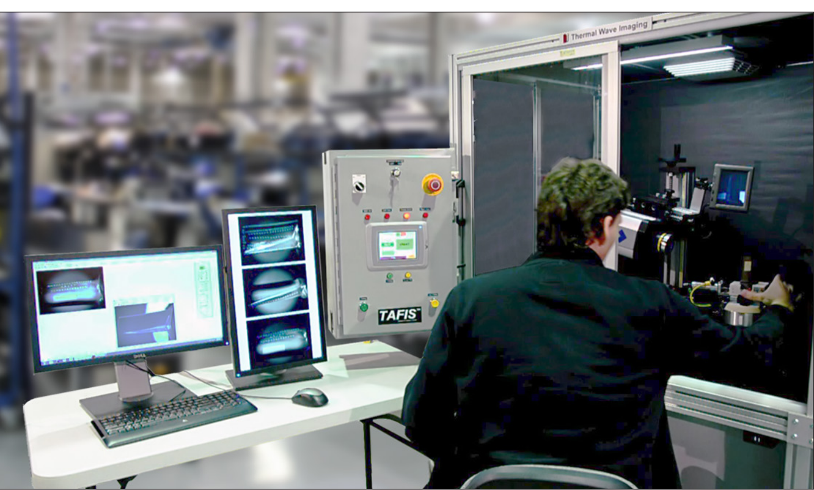
A TAFIS inspection station, for cooling hole blockage detection in turbine engine blades, operates on TWI's plant floor.
