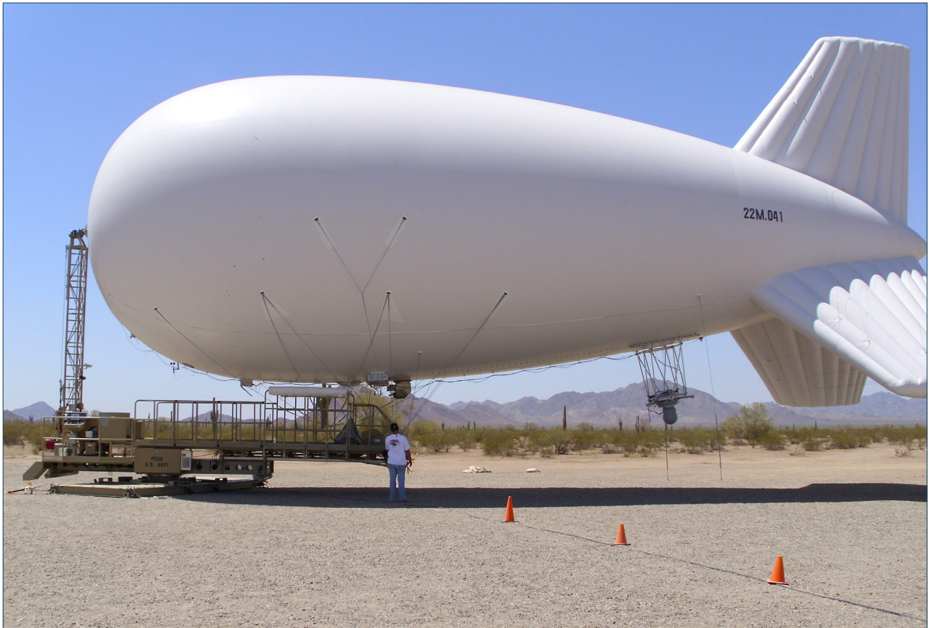
The one-fiber, multi-radio system known as HARC uses tethered “eye-in-the-sky” aerostats to position the hardware.
