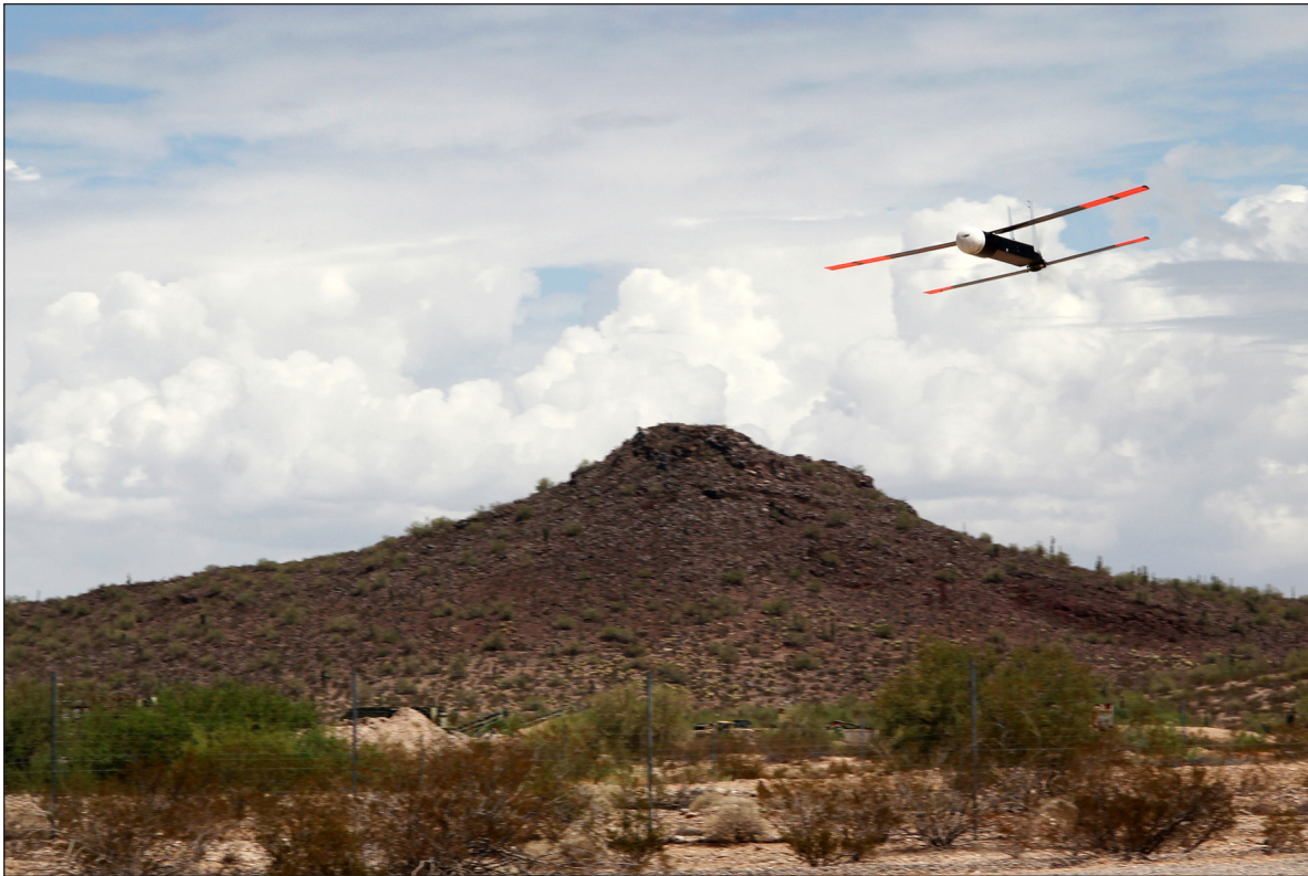
The coyote unmanned aircraft system is used by the National Oceanographic and Atmospheric Administration for hurricane tracking.
